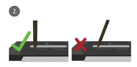
ALIGN INDICATOR LINE ON STAMP WITH LINE ON JIG AND AIM TO FORM A 90 DEGREE ANGLE. ENSURE BOTH LINES TOUCH - NO GAPS.
