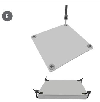
CORNER HOLES CAN BE USED TO SECURE TO A SURFACE USING SCREWS/NAILS, OR STACK MULTIPLE PLATES TOGETHER WITH LOCKS, ZIP TIES, OR HARDWARE (NOT INCLUDED).
