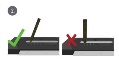
ALIGN INDICATOR LINE ON STAMP WITH LINE ON JIG AND AIM TO FORM A 90 DEGREE ANGLE. ENSURE BOTH LINES TOUCH - NO GAPS.
